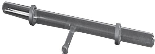
The discharge tube is for observing light produced during electrical discharges in gases at reduced pressure and for studying cathode and canal rays that are observed outside the path of the discharge at low pressure.
