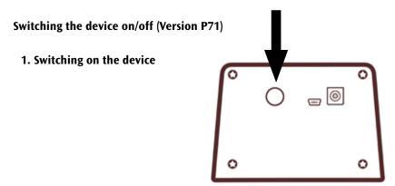
The electronics inside the  $CPRLilly^{TM}$  automatically switch off after 5 minutes of inactivity, or the device can be switched off manually by holding down the on/off button.
