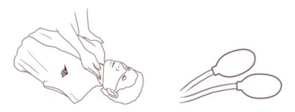
The pulse can be adjusted with the white squeeze ball (P70) or via the software (P71).
