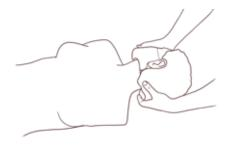
To free the airways, the simulator head can be rotated by 90°.
