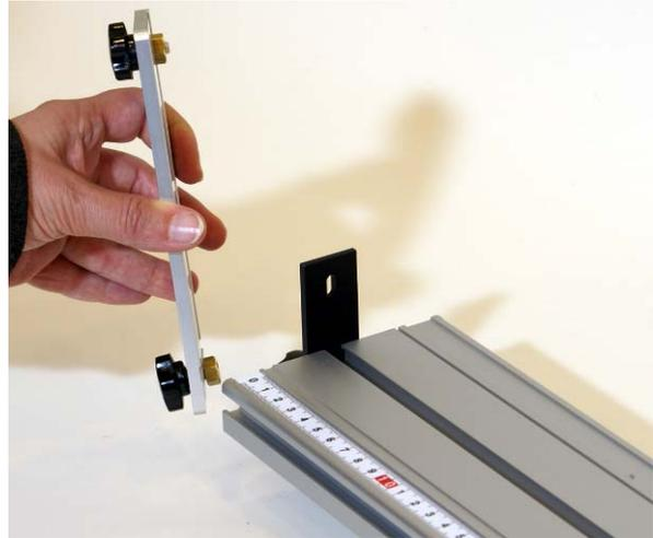
Fig. 16 Inserting the holder for light barrier into the groove at the side of the trolley track
