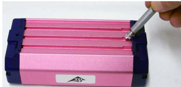
Fig. 24 Inserting the contact-breaker into the groove on the upper side of the trolley
