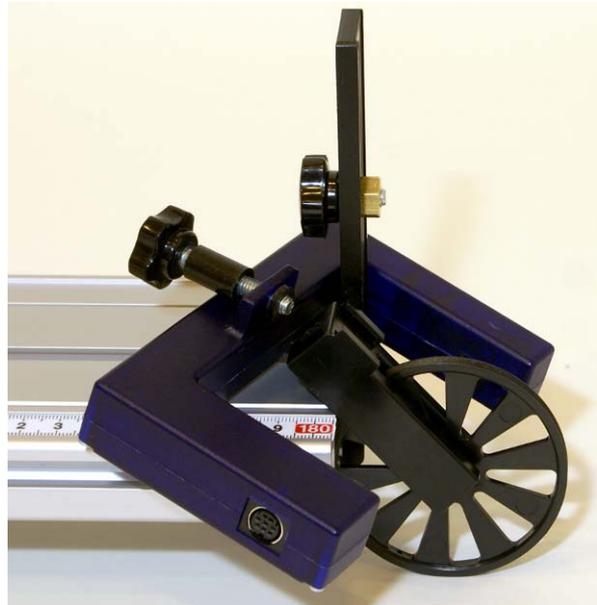
Fig. 11 Set-up of pulley on light barrier
