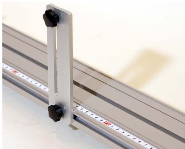
Fig. 17 Mounted holder for light barrier
