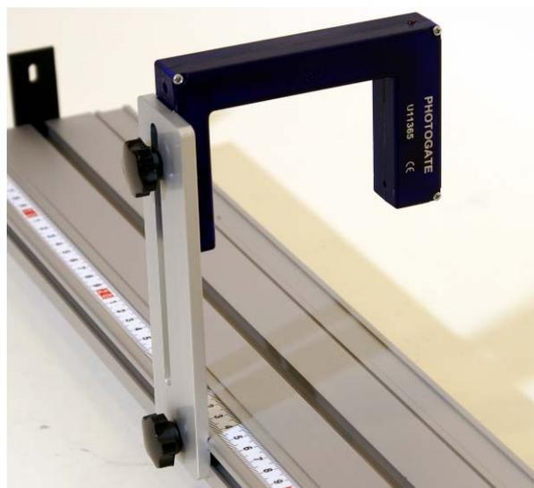
Fig. 18 Mounted light barrier
