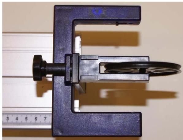
Fig. 12 Complete set-up for light barrier and pulley
