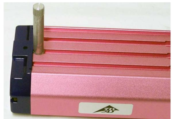
Fig. 25 Mounted contact-breaker
