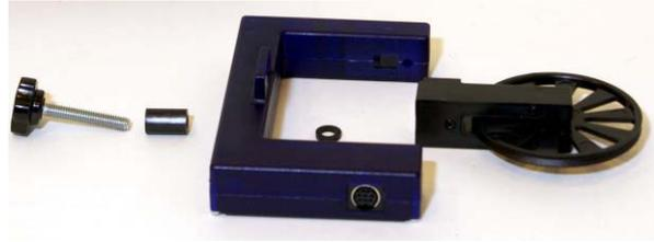
Fig. 10 Photoelectric light barrier and pulley
