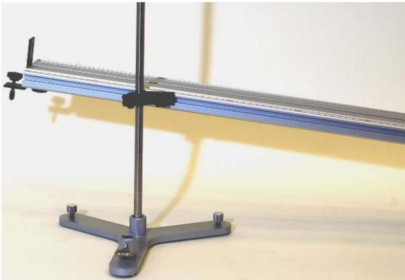
Fig. 20 Completed mounting of clamp for rods in the groove at the side of the trolley track
