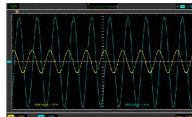
Fig. 1: Coil in an AC circuit: Current and voltage over time
