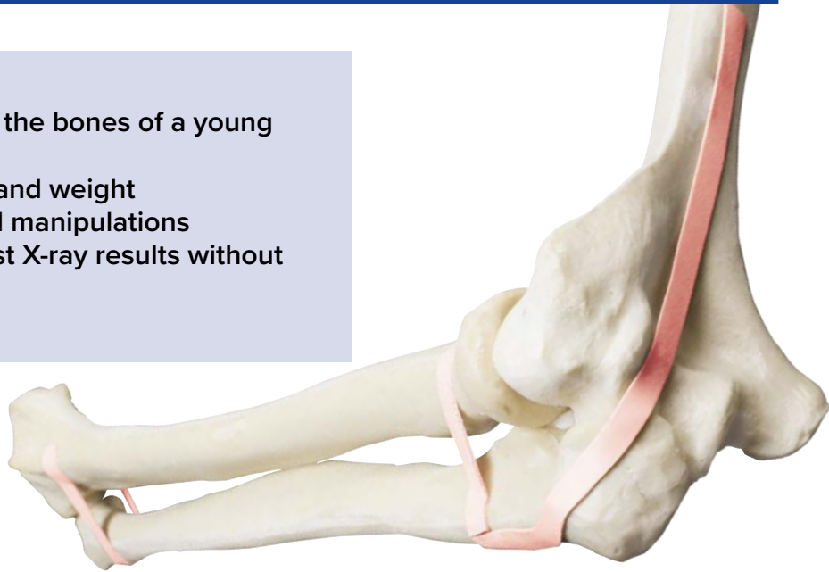
Latex bands simulate joint movement and leave no trace on the X-ray
