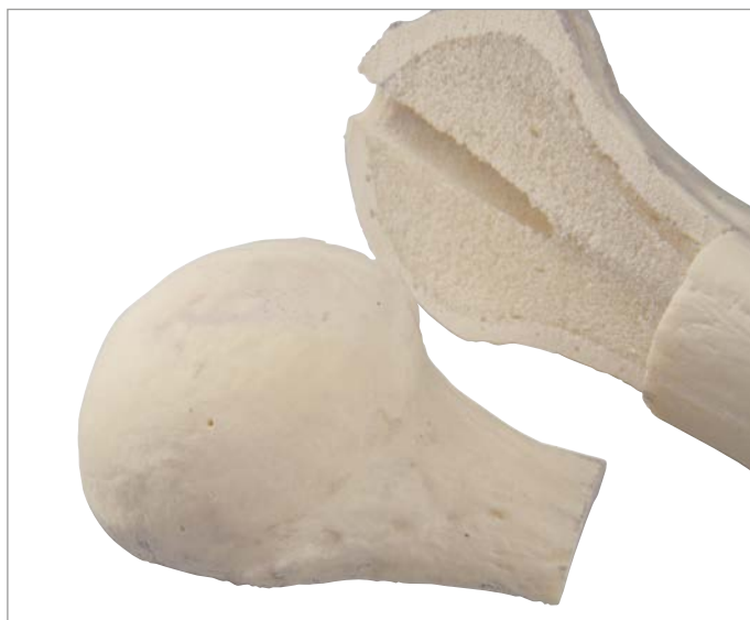
The multilayered construction simulates the hard cortical and the softer cancellous bone. Mechanical manipulations (i.e. with screws, plates, or implants) can be practised on these highly realistic workshop bones.
